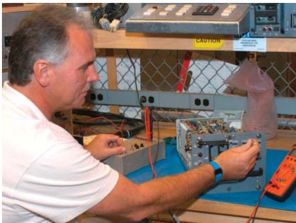
Bruce Telincho, a Pittston Township resident, tests a telephone circuit switch power supply component at Tobyhanna Army Depot. The component will be used in AN/TTC-46 and 47 Mobile Subscriber Equipment. (by Anthony Ricchiazzi)
