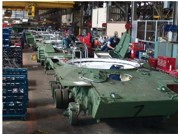
Four M-1 Abrams tanks are in various stages of upgrade on the reassembly line at Anniston Army Depot Combat Vehicle Facility.
