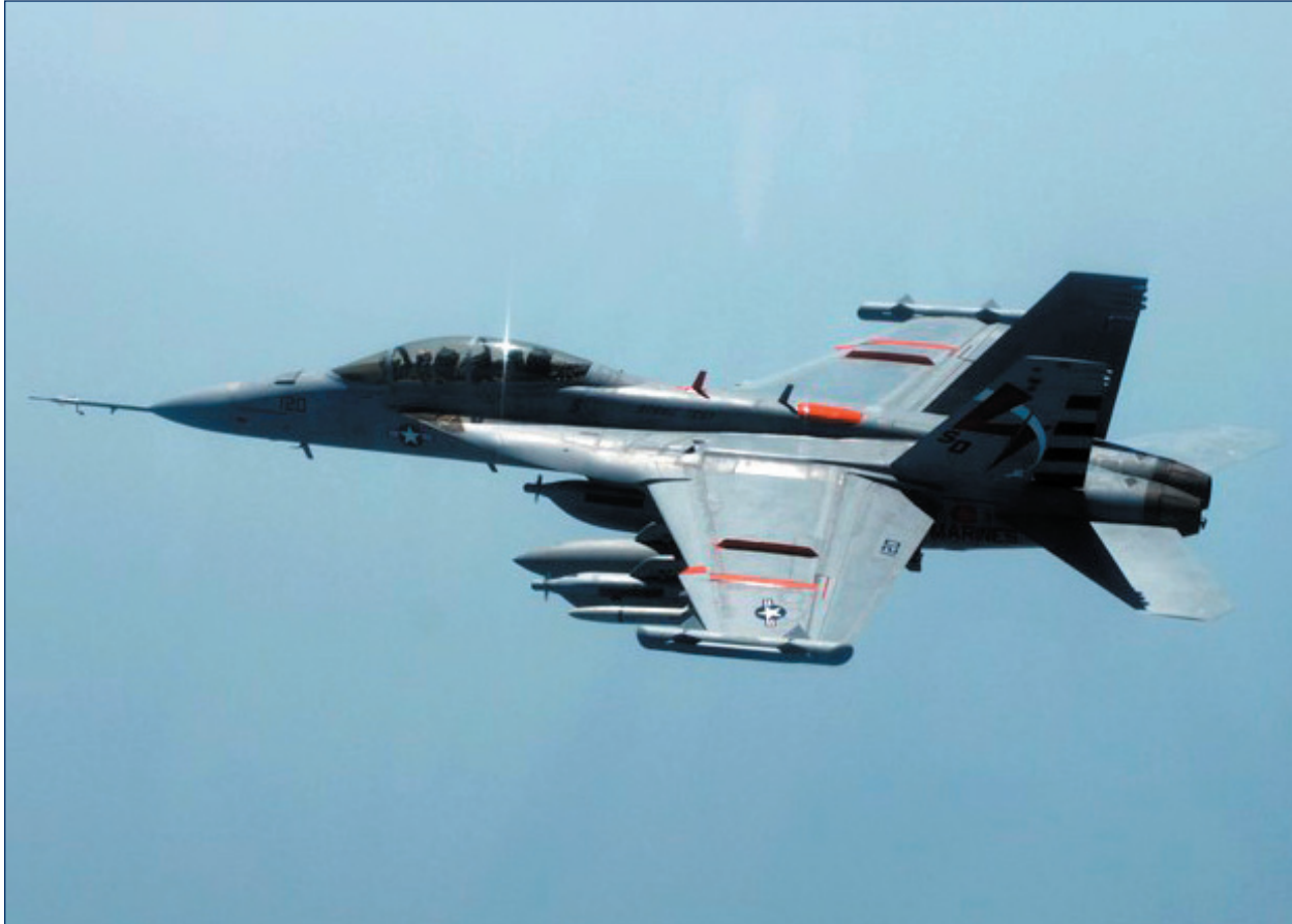
The EA-18G Growler, the Navy's next-generation electronic attack aircraft, is being developed to replace the fleet's current carrier-based EA-6B Prowler. The EA-18G is expected to enter initial operational capability in 2009.
