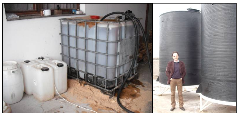
Bio King collects used oil in the small containers shown in the left photo, then filters it into the square intermediate bulk container (IBC). The temperature must be sufficiently high to pump the oil so filtration is done indoors. The filtered oil is then pumped into the outside storage tanks for pickup; at the time of the interview Mr. Nestic had 16 tons in the tanks awaiting pickup. He has already provided 4000 L of used oil to his buyers. In Belgium, Mr. Nestic visited a company of only four employees that collects 6000-8000 ton/year.
