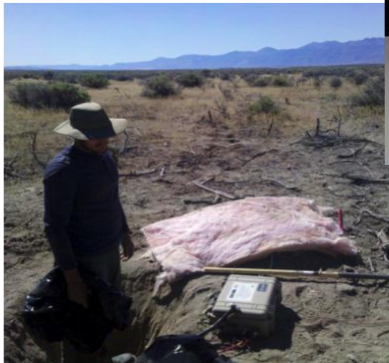
Zonge wideband EM receiver with three-component magnetic field sensor and OSU-fabricated electrodes used to sense electric fields.
