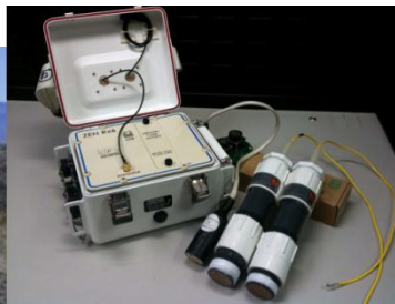
Zonge wideband EM receiver with three-component magnetic field sensor and OSU-fabricated electrodes used to sense electric fields.
