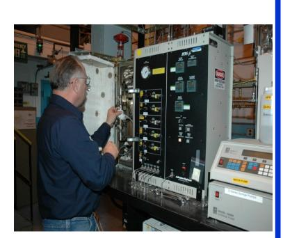
Our reactors can test many impurities including HCl, H<sub>2</sub>S,  $SO_2$ , and  $NO_x$
