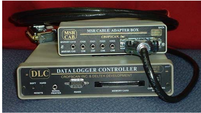
Figure 64. data logger controller & cable adapter box
