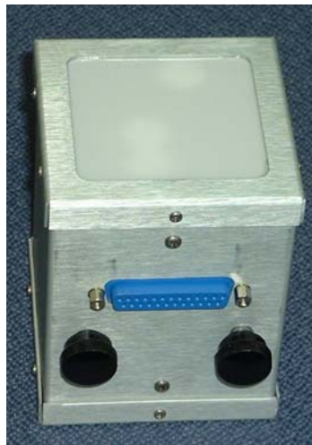
Figure 63. CROPSCAN Multispectral Radiometer (MSR). (Size is 8 X 8 X 10 cm)
