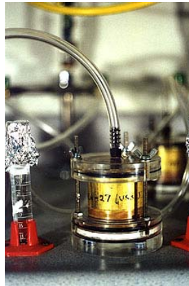
Figure 36. Example of experimental setup for water retention curves from soil cores using Tempe cells.
