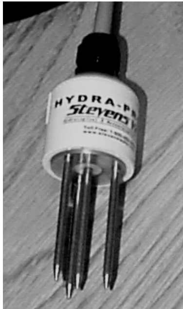
Figure 59. The Hydra probe used at the tower locations.
