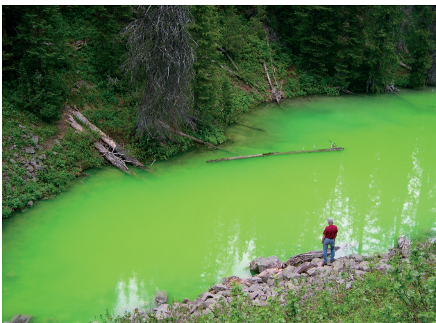
Mammoth Crystal Springs about 24 hours after green (fluorescein) dye tracer test, Yellowstone National Park (David Susong, USGS, 2005).
