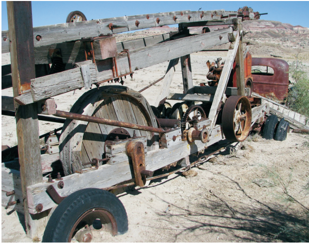
Cable tool water well drilling rig in the backcountry of Capitol Reef National Park (Phil Ayers, IMR, 2007).
