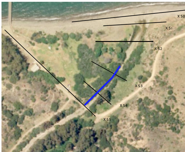
Figure 1. Overview photo of the lower reach of Cañada del Puerto Creek, Santa Cruz Island. The approximate location of the channel and floodplain cross sections are depicted as black lines and labeled XS0 through XS5. The thick blue line is the approximate location of the left bank levee (Noon, 2006).
