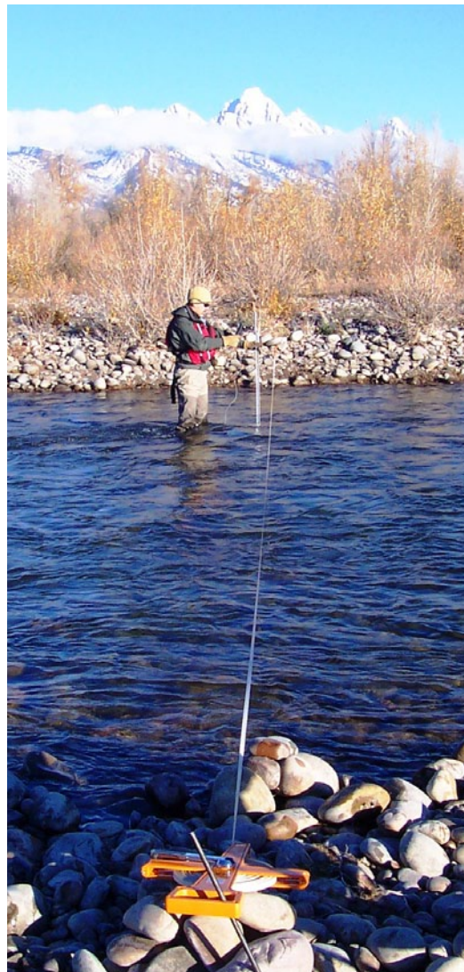
Discharge measurement on the lower Gros Ventre River, Grand Teton National Park (Wyoming). NPS/GWEN GERBER
