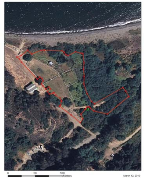
Aerial photograph of Prisoners Harbor with surveyed boundary of the proposed restoration area. Green points are recoverable reference points.
