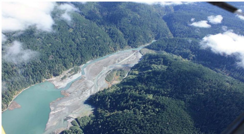
Lake Mills delta and Elwha River, November, 2010. Notice: 1) most river flow is in the recently constructed center channel, 2) "bathtub" ring in the lake is due to reservoir draw down, and 3) active erosion and redistribution of delta sediments. (Photo by NPS)
