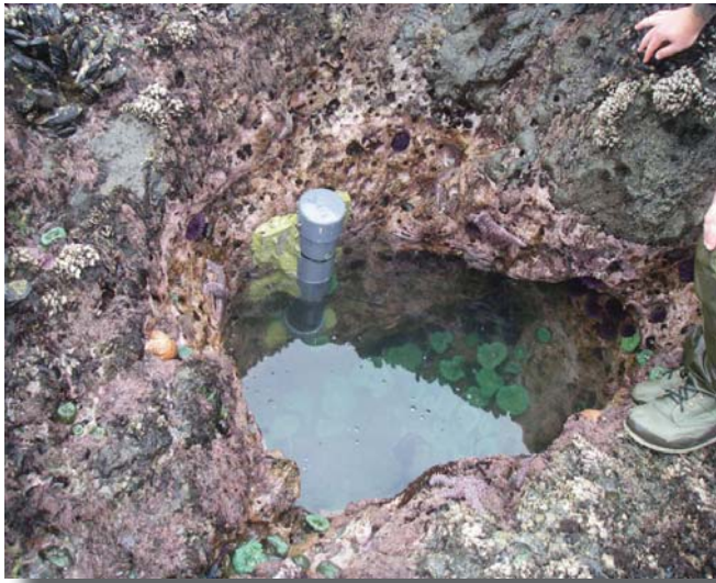
Housing for a multiprobe datasonde to monitor ocean acidification in a low elevation tidepool at Sokol Point, Olympic National Park (NPS Photo Credit: Steve Fradkin); Housing containing a multiprobe data sonde to monitor ocean acidification in a low elevation tidepool at Brown's Point, Olympic National Park. (NPS Photo Credit: Steve Fradkin)
