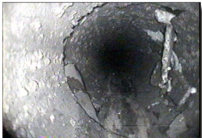
Pre-closure, downhole video of break in casing thermal well in Yellowstone National Park (NPS 2008).
