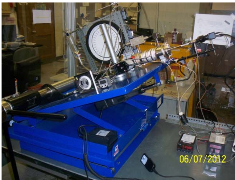
Figure 12: Experimental setup of the HTHP rolling ball viscometer.
