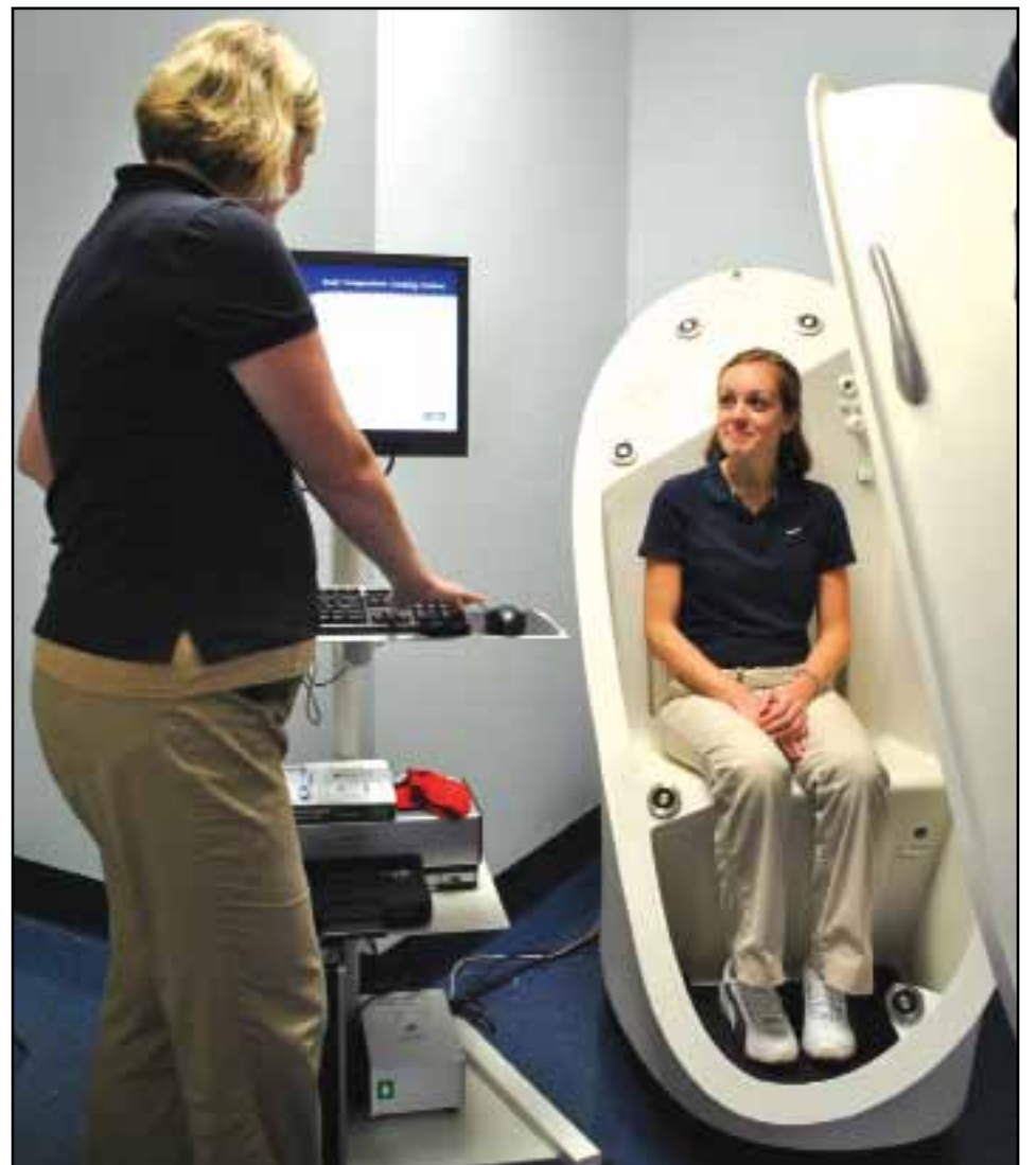
Sarah Fewell and Sarah Guin, health educators at the Fort Bragg Army Wellness Center, demonstrate the Bod Pod, which measures the ratio of lean muscle mass to fat in five minutes, rather than 45 minutes needed for hydrostatic measuring.
