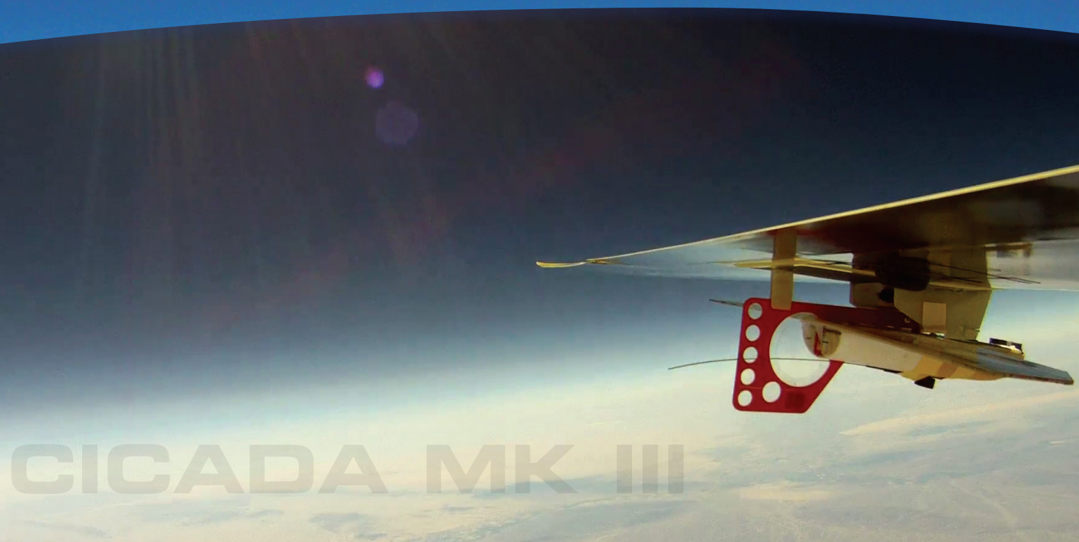
A CICADA Mark III is carried beneath the left wing of the Tempest UAV at 53,000 feet, after release from the balloon and before releasing the CICADA.
