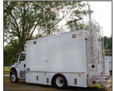
The USAPHC Mobile Ambient Air Monitoring System vehicle is capable of rapid deployments and is often used to monitor air quality. (Photo by Christina Graber)
