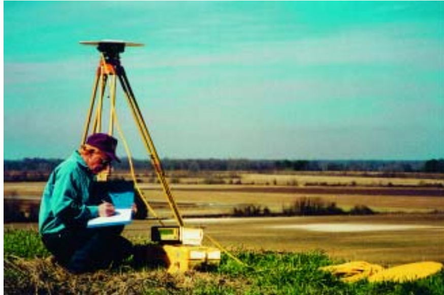
Figure 7-2. Typical ground receiver data collection
