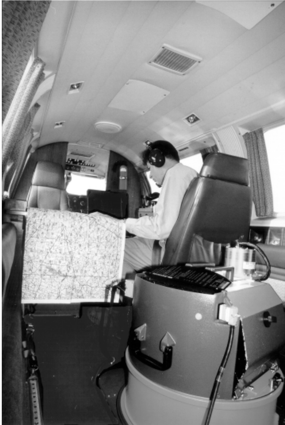
Figure 5-2. Typical camera system mounted in an aircraft (Courtesy of Dave Kreighbaum and Earthdata Corporation)
