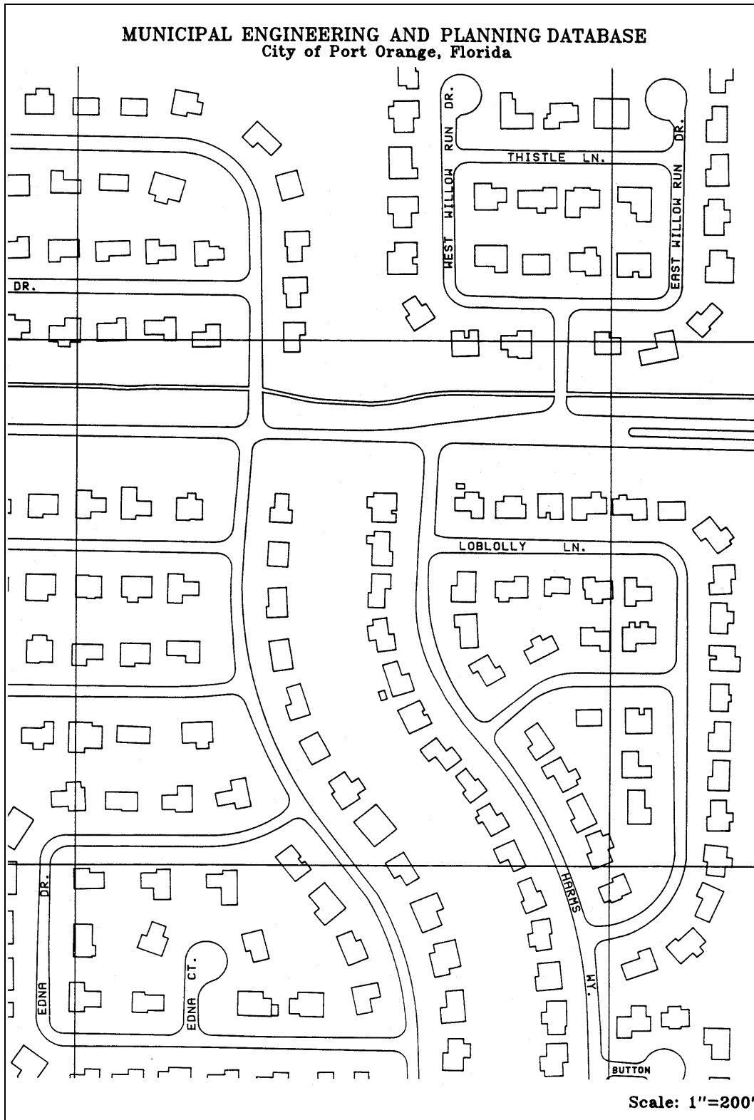
Figure 4-3. Planimetric map of residential area, 1-in. = 200-ft scale, for general planning purposes (Courtesy of Southern Resource Mapping Corporation)
