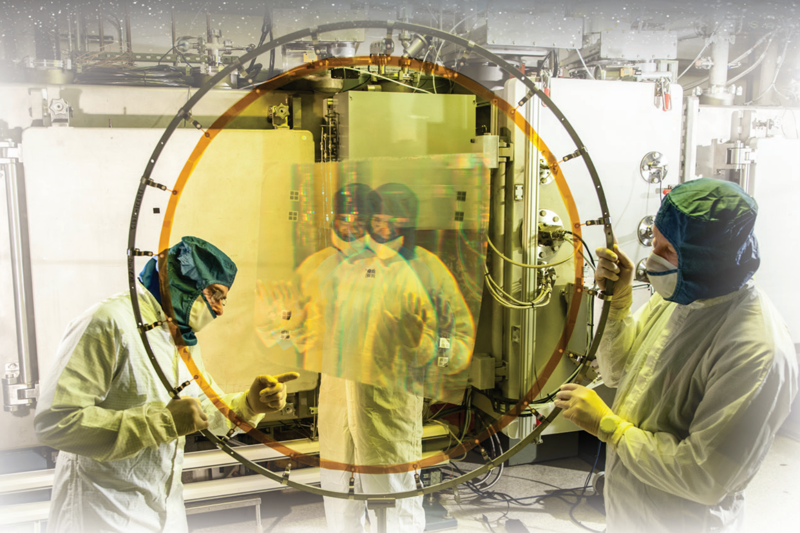
Lawrence Livermore, Ball Aerospace and Technologies Corporation, and NeXolve Corporation are preparing diffractive membrane optics for the Membrane Optic Imager Real-Time Exploitation (MOIRE) project.
