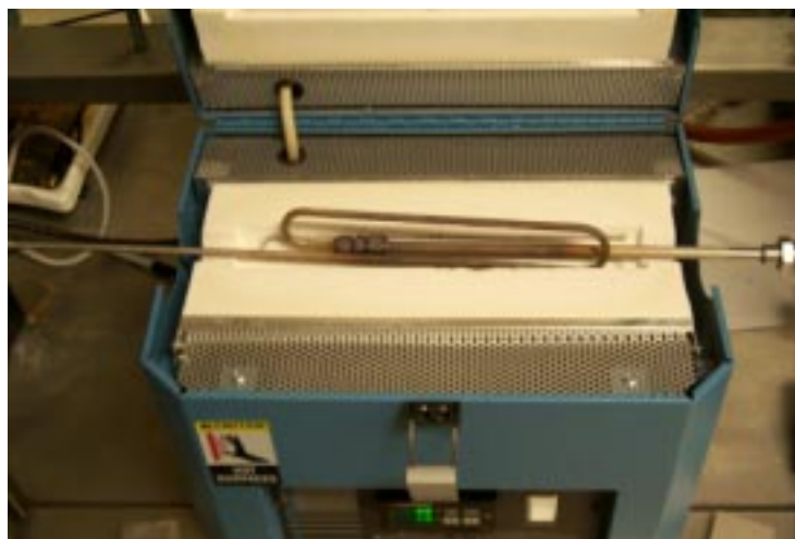
Figure 4. Photo of heat exchanger
