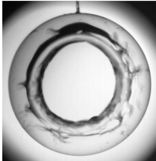
FIG. 8: The HD ice before IR layering. The ice moved to the relatively cooler center of the shell overnight due to room light entering the hohlraum. The ice returned to nearly the same shape every night.
