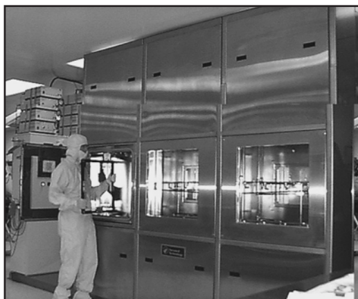
FIGURE 6. Optic being loaded into the Forward Technology Industries automated solvent cleaning system. (40-00-0600-2889pb01)
