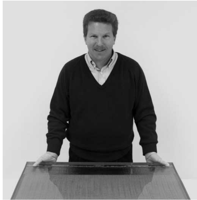
FIGURE 1. NIF-size laser glass slab from Schott's 1998 development campaign. (70-00-0198-0098pb01)
