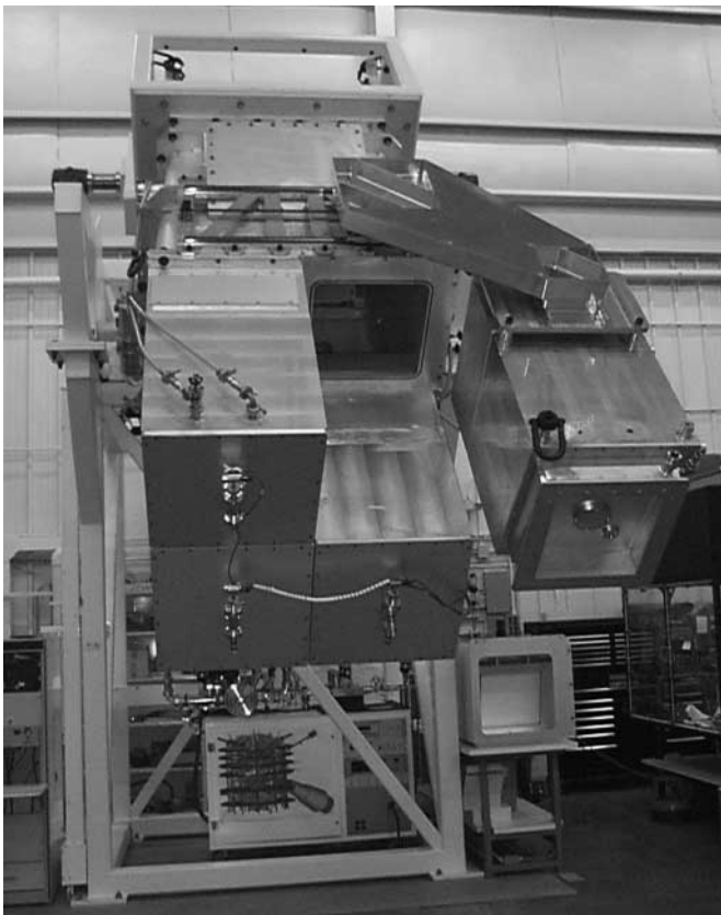
FIGURE 5. IOM 2-dof fixture with IOM in fully retracted position. (40-00-0199-0195pb01)
