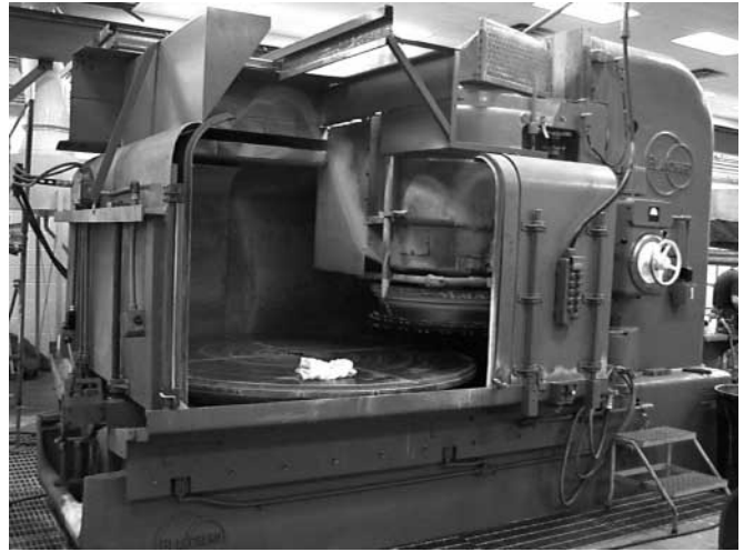
Blanks ground to final size on Blanchard (from Oak Ridge)
