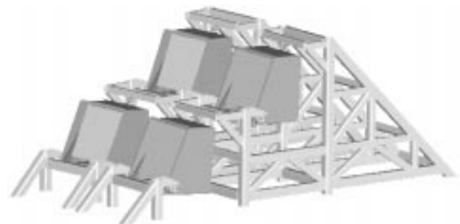
FIGURE 20. Typical mirror structure with transport mirror modules. (40-00-1097-2288pb01)
