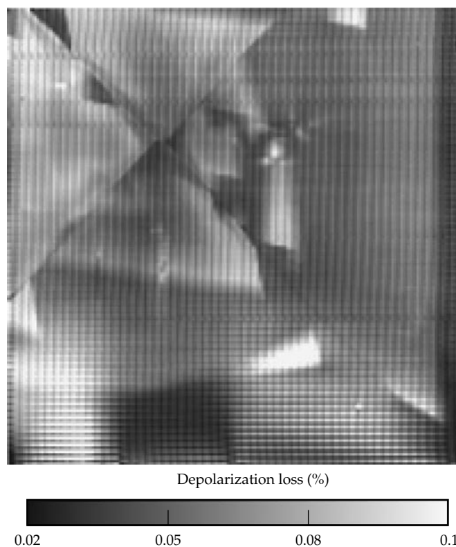
FIGURE 7. Photograph of DKDP crystal with the deuteration level about 92%. The size in cross section is 50 × 50 cm 2 . (40-00-0697-0987pb01)
