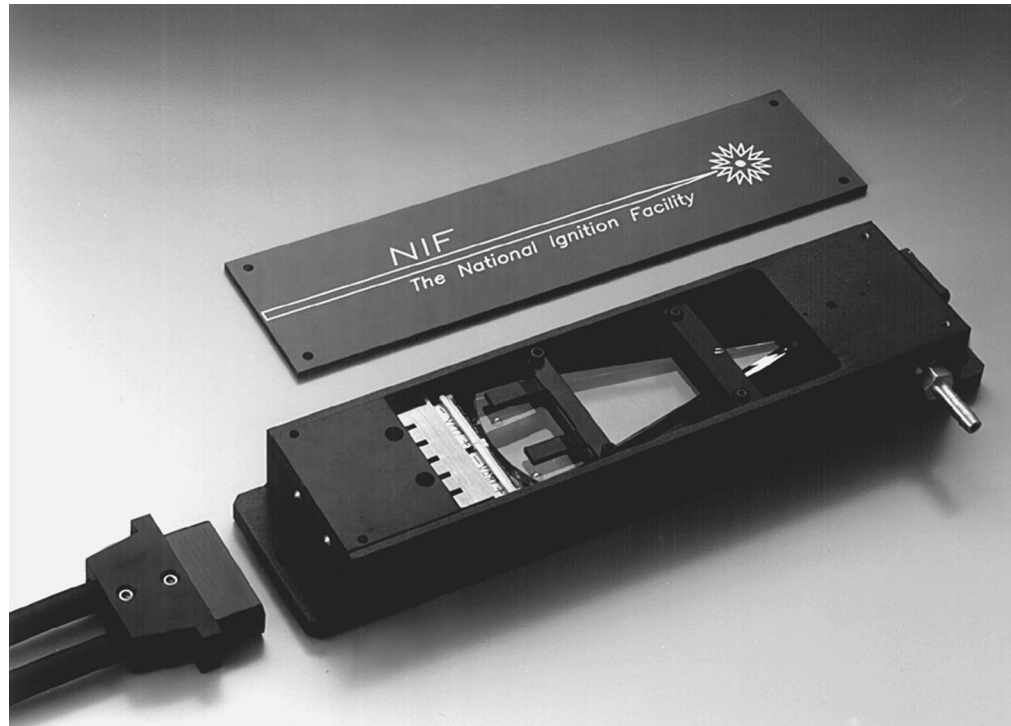
FIGURE 6. Photograph of a NIF regenerative amplifier head illustrating the compactness of a lens duct and laser diode array. (99-00-0595-1337pb02)
