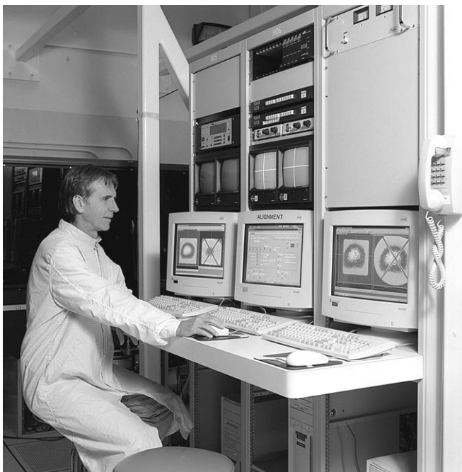
FIGURE 8. Control console for U.S.-French large-aperture diagnostic system. (70-00-1197-2406pb01)
