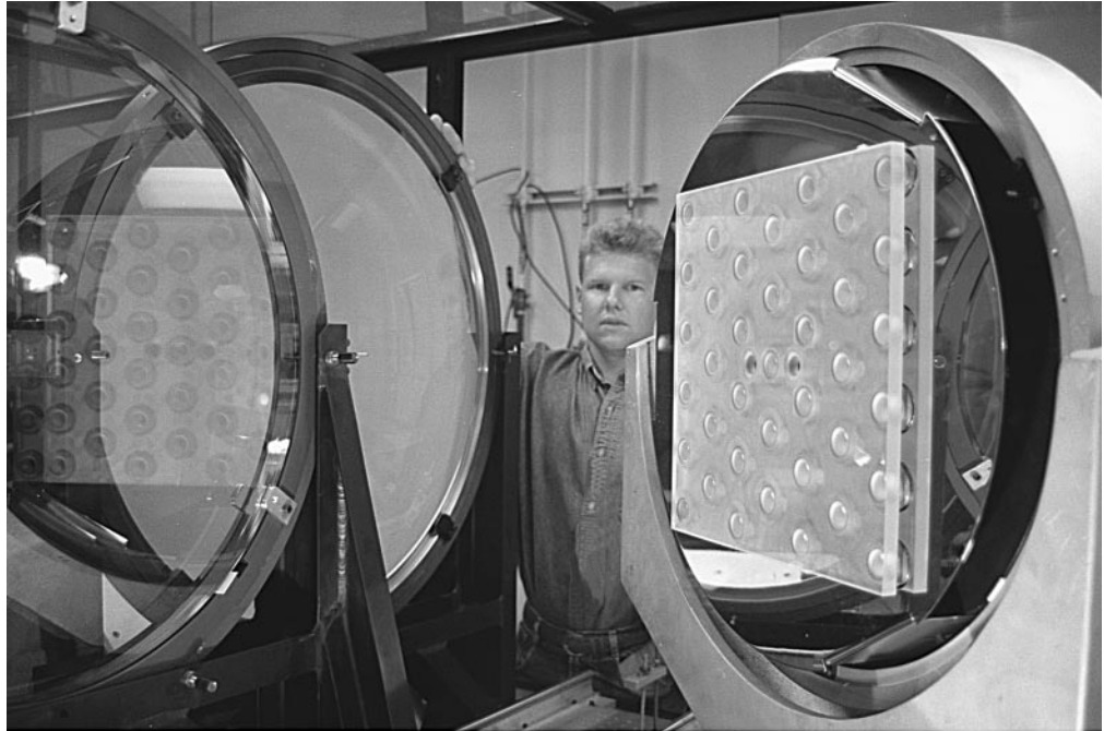
FIGURE 11. A 40-cm deformable mirror. (02-01-0897-1511#22pb01)
