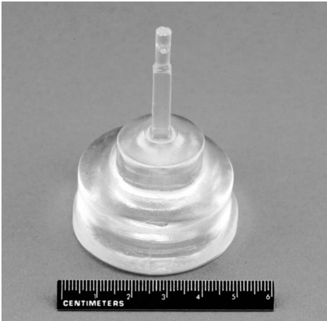
FIGURE 16. Photograph of an Yb:S-FAP laser crystal and laser diode array tile. (70-17-0695-1699Cpb01)
