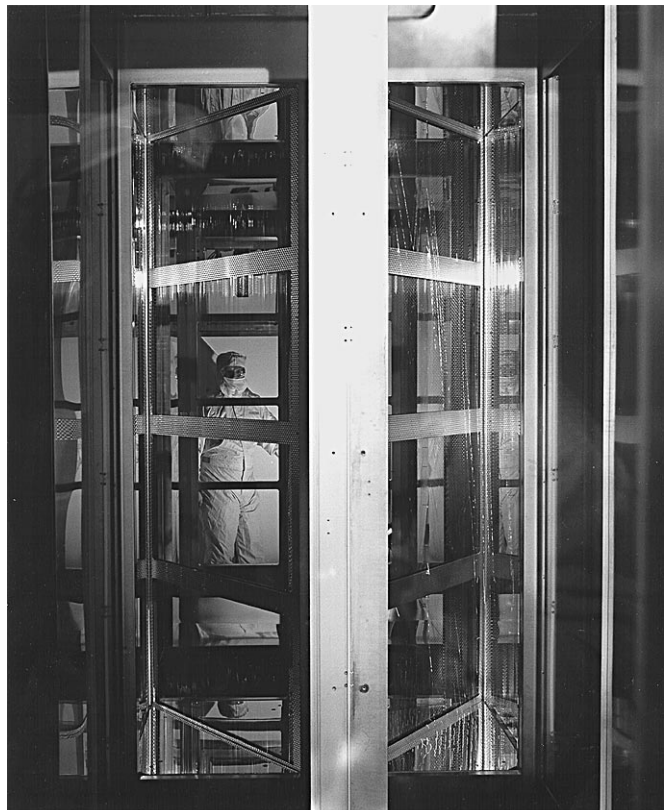
FIGURE 7. NIF prototype amplifier under test in AMPLAB. (70-00-0997-1885#9pb01)
