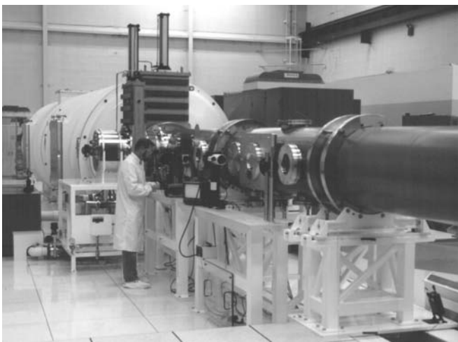
FIGURE 3. A vacuum test station added to Beamlet to evaluate the focusing properties of the beam after conversion to the third harmonic. (70-50-0496-0721pb01)
