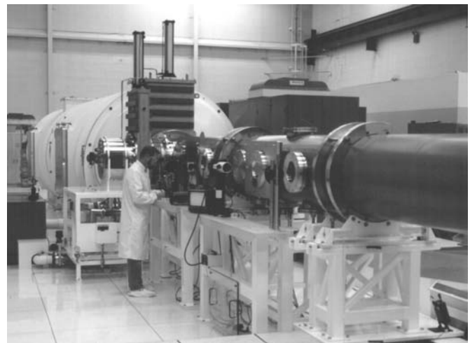
FIGURE 4. The 100-TW laser installed on the Nova 2-beam chamber. (70-60-0895-1969Apb01)
