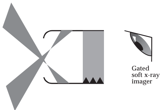
FIGURE 14. Experimental geometry for viewing rippled wall. (NIF-0403-06140pb01)
