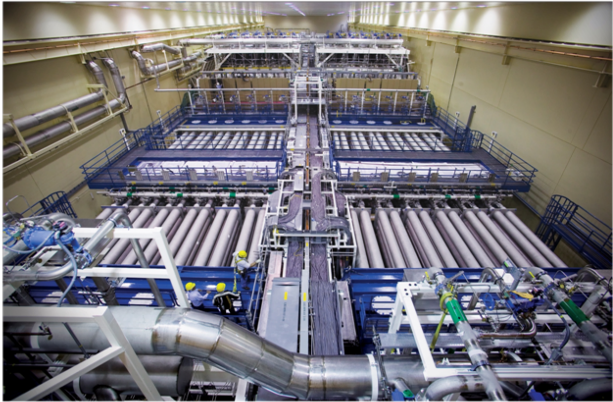
Figure 4. Photograph of one of the two laser bays of the NIF; note the workers in the lower left corner for scale. Each bay accommodates half of the 192 individual laser beams that comprise the NIF laser system. The \sim 40 \times 40 cm aperture laser beams are transported in large diameter pipes clearly visible in the photo. The main laser amplifiers are assembled in the laser bay at given positions along the beamlines.
