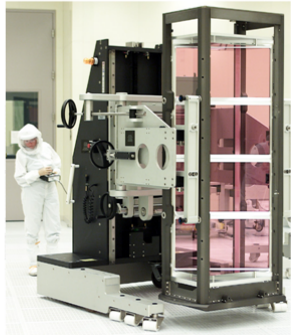
Figure 5. (a) Precision laser glass plates are assembled in (b) cassettes for installation on the NIF. A total of 768 such cassettes are used in the NIF amplifiers.
