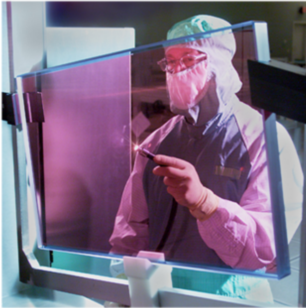
Figure 5. (a) Precision laser glass plates are assembled in (b) cassettes for installation on the NIF. A total of 768 such cassettes are used in the NIF amplifiers.
