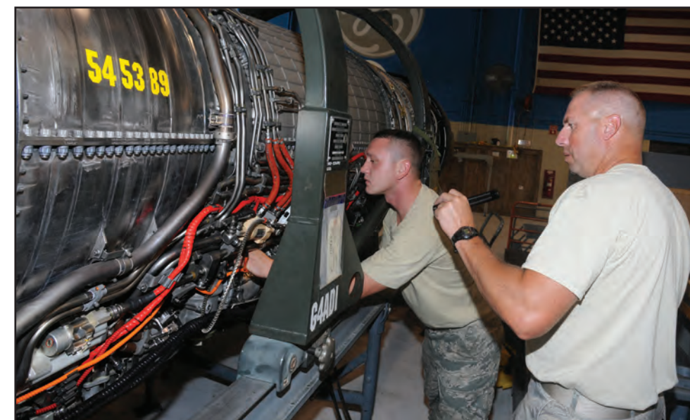
Master Sgt. Mark Lueth oversees a feedback cable replacement by Senior Airman Jonathan Baumgartner during the August Unit Training Assembly at Joe Foss Field
