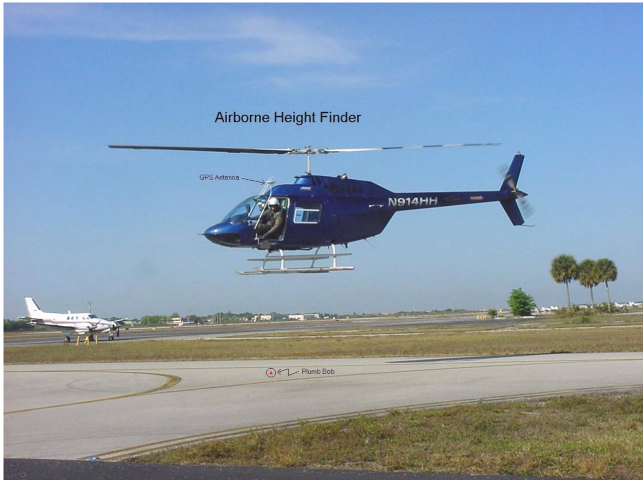
Figure 2. Pre-mission testing of the AHF just following lift-off. The operator calibrates and drops the plumb-bob from the leveling plate and when the cable reaches a specified resistance, the global positioning system (GPS) captures the horizontal and vertical position. Post-processing yields vertical accuracies that are better than +/- 15cm.
