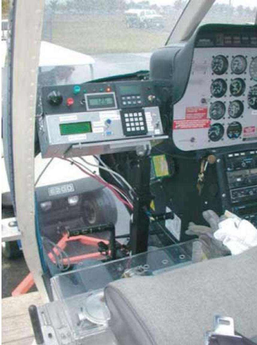
Figure 1. The airborne height finder (AHF) system as installed in a helicopter. The system control panel is evident in the center of the photograph. The plate and plumb-bob system reside just forward of the seat.
