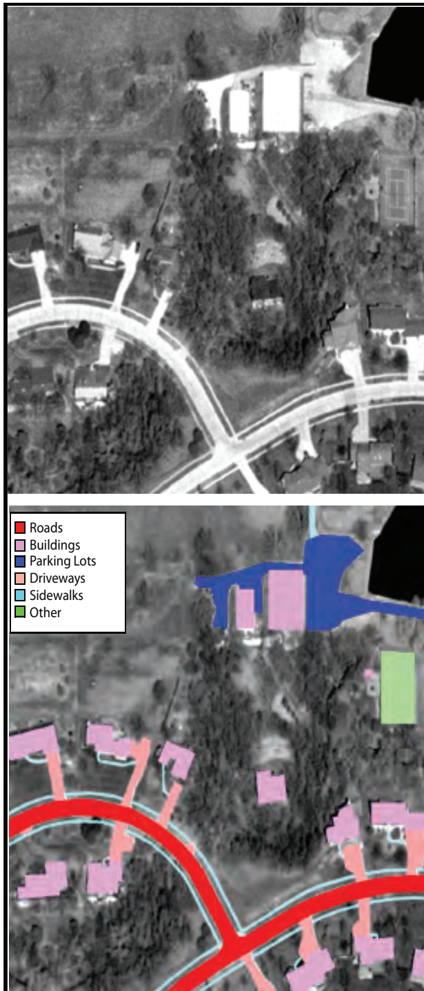
Figure 2. An example of heads-up digitizing of six classes of impervious-surface from rectified high-spatial-resolution imagery.
