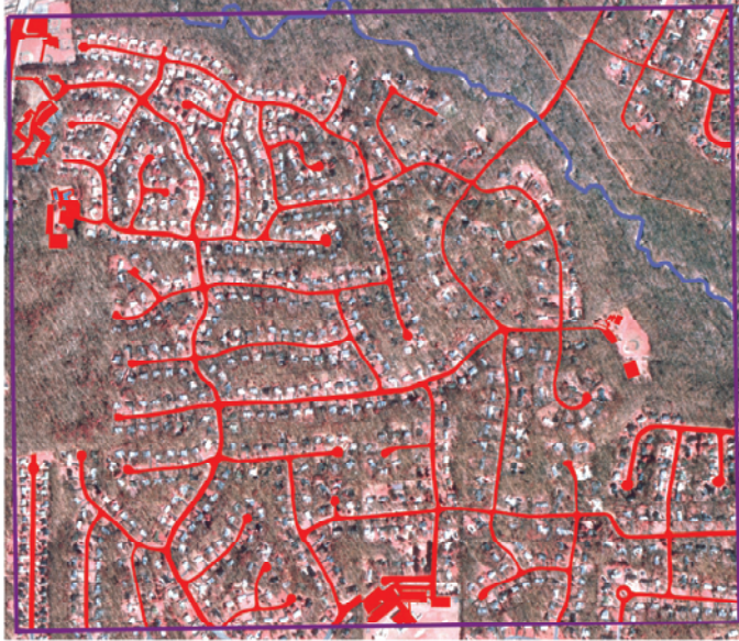
Figure 3. Direct impervious-surface compilation method. Delineated roads, parking lots, and commercial/institutional rooftop areas are mapped in red. Accotink Creek is mapped in blue.
