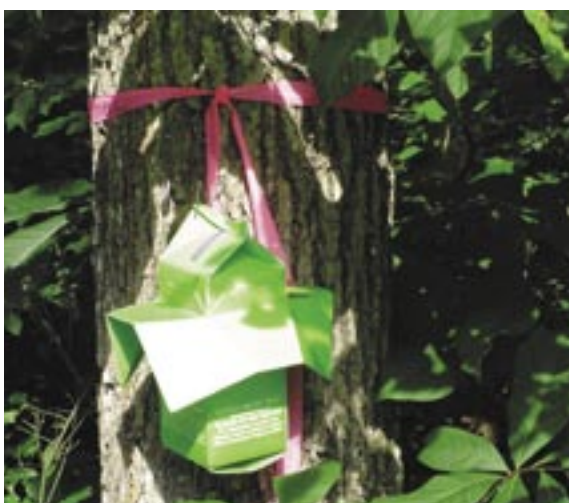
A milk carton trap used to sample male response to the gypsy moth female sex attractant (pheromone).
