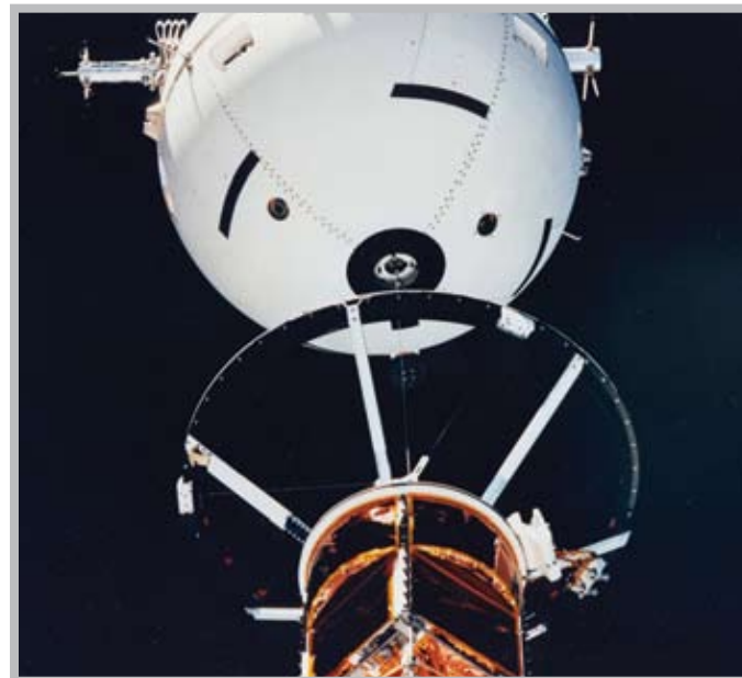
Onboard view of the early operations with the Tethered Satellite System [TSS-1]. The sphere will move away from the ring structure on the boom device. [NASA/KSC Digital – Archives]
