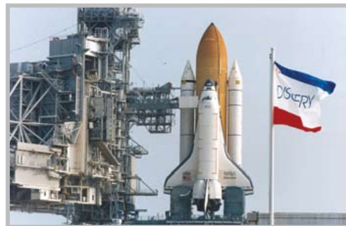
Preliminary reports indicate the Space Shuttle's first super lightweight external tank (SLWT) is in excellent condition following the completion of a tanking test yesterday. [NASA/JSC Digital]
