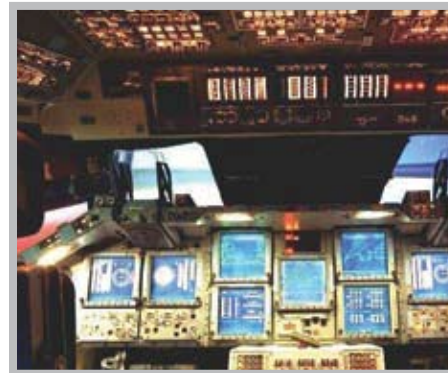
This image illustrates NASA's Multifunction Electronic Display Subsystem (MEDS), otherwise known as "glass cockpit." [NASA/JSC Digital]
