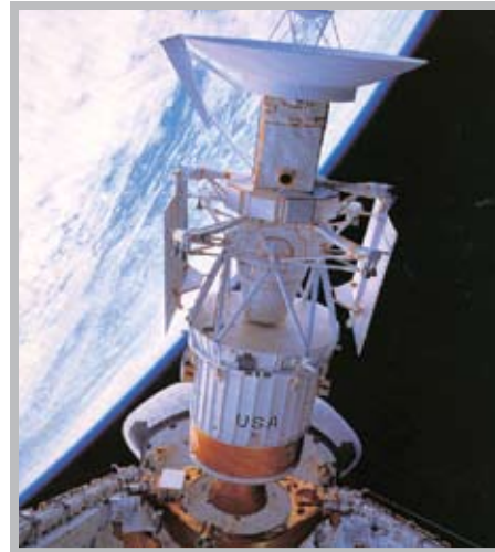
Inertial upper stage (IUS) with Magellan spacecraft is deployed from the payload bay (PLB) of Atlantis, Orbiter Vehicle (OV) 104, during STS-30. [NASA/JSC Digital]
