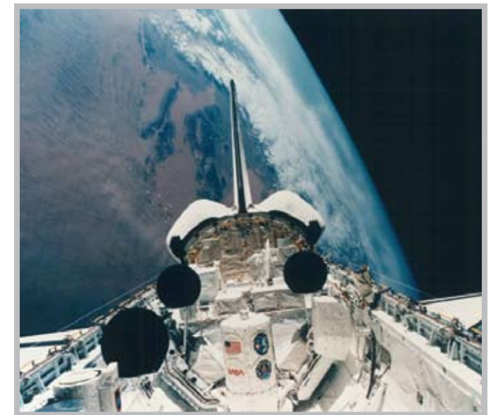
ATLAS-1 in space inside cargo bay of Atlantis. Also visible is a single Get Away Special and the Shuttle Solar Backscatter Ultraviolet/S. [NASA/KSC Digital – Archives]
