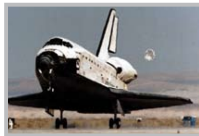
The drag chute on the Space Shuttle Discovery begins to unfurl as the vehicle rolls toward mission completion at Edwards Air Force Base. [NASA/JSC Digital]
