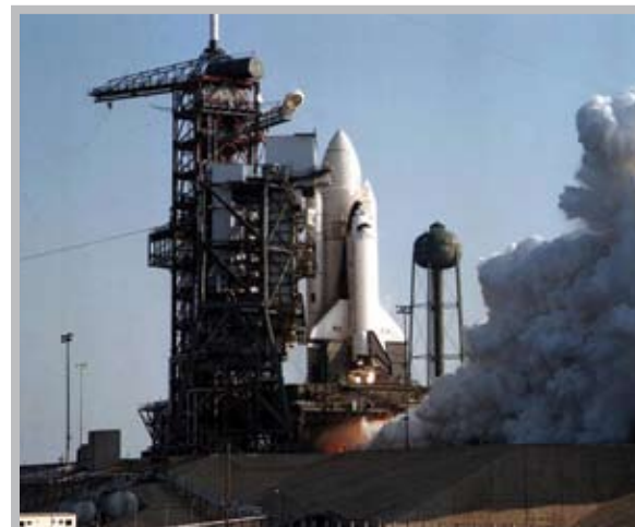
STS-1 Static Firing of the Space Shuttle's three main engines overall view at Complex 39A [NASA/KSC Digital - Archives]
