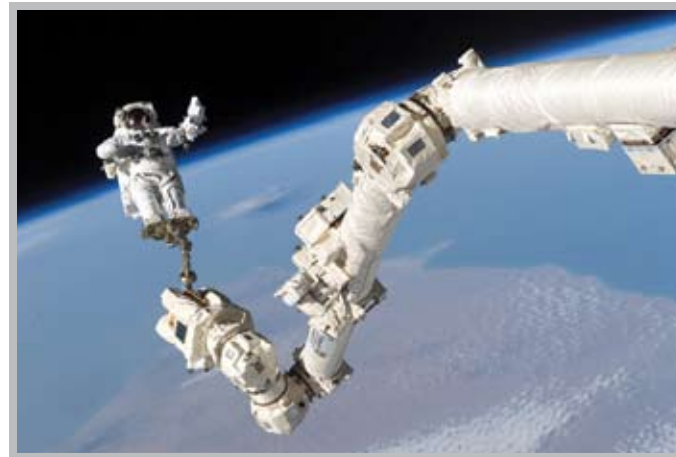
A camera attached to the space shuttle Discovery's robotic arm shows astronaut Steve Robinson going under the underside of the Discovery to remove gap fillers in this view from television Wednesday, Aug. 3, 2005. This is the first time in spacewalking history that an astronaut has ventured under the belly of a space shuttle and performed repairs. [NASA/KSC Digital]
