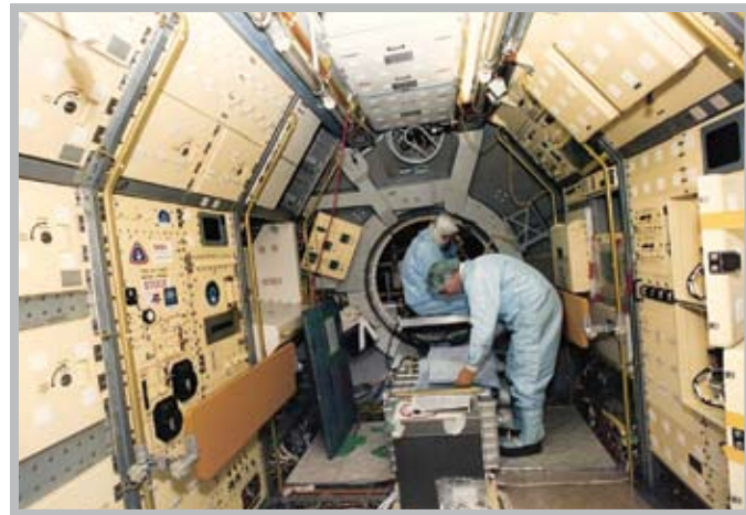
Clean-suited crewmembers and technicians examine and test USML-1 spacelab (SL) module systems during preflight procedures in Operations and Checkout (O&C) Building. [NASA/JSC Digital]
