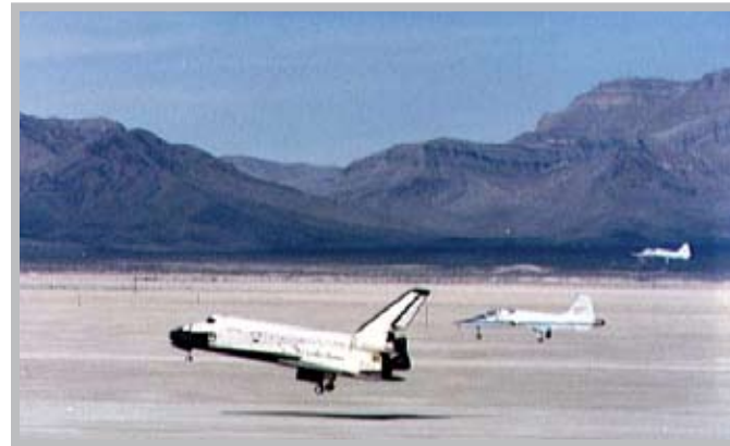
Columbia is shown seconds from touchdown with two T-38 chase planes following it in to the landing strip. [NASA Digital]
