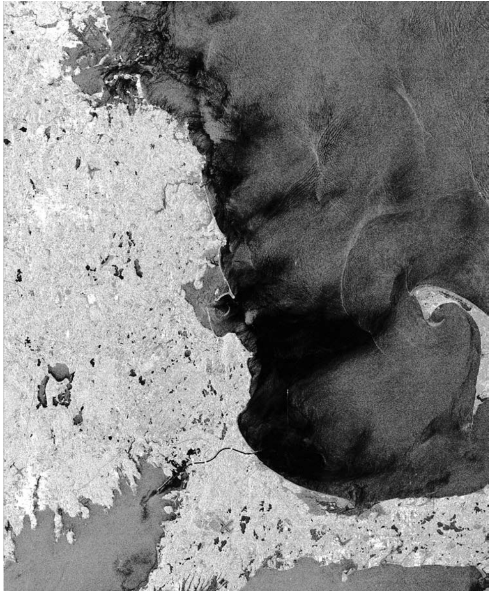
Three internal wave packets are obvious as curvilinear features in the sanctuary area north of Cape Cod. Image courtesy of European Space Agency, processed by Jose da Silva, Univ. of Lisbon. Envisat ASAR, 7 August 2003 2:30 GMT; image precision mode.
