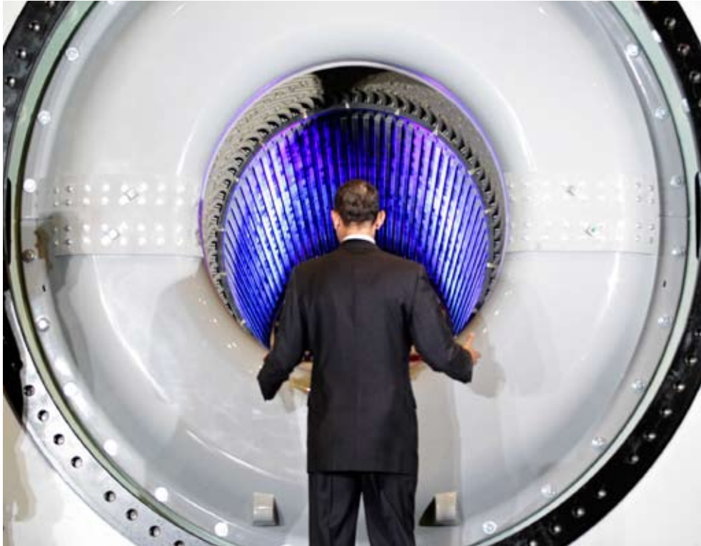
President Barack Obama inspects a hydrogen-cooled generator being manufactured for a power station in Kuwait at a General Electric plant in Schenectady, New York.
