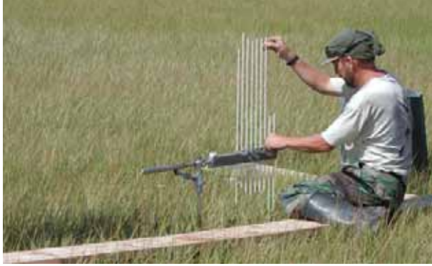
Elevation change can be monitored with surface elevation tables placed on benchmarks installed in wetlands.
