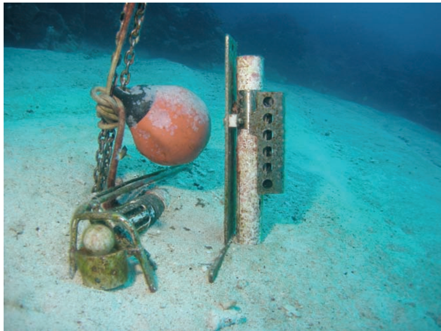
Figure 19. The YSI and Seabird water quality instrument partially buried in sandflat at buoy #2 on WFGB (October 2008).
