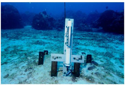
Seabird water quality instrument mounted on rack in sand at East Flower Garden Bank. This instrument measures temperature and salinity. The instrument rack has been partially buried by sand shifting as a result of Hurricanes Rita (2005) and Ike (2009).
