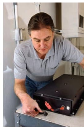
Experimental lithium ion battery for hybrid-electric cars capable of getting 100 mpg. DOE/Sandia National Laboratories
