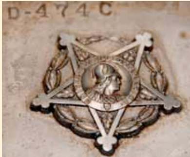
TIOH keeps an archive of hubs and dies for medals they design. The Medal of Honor hub is pictured.
