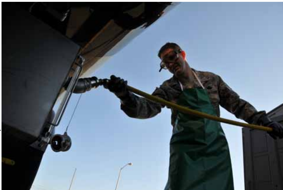
Master Sgt. William Frederick, 934th Airlift Wing fuels superintendent, pours an anti-icing additive into a fuel truck as part of the AFSO21 "JP-8 to Jet A fuel conversion" demonstration at the Minneapolis-St. Paul Air Reserve Station, Minn. on Nov. 17. (Air Force Photo/Tech. Sgt. Jeffrey Williams)
