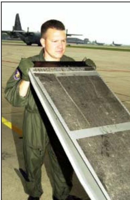
Staff Sgt. Patrick Haley, 96th Airlift Squadron loadmaster, closing the auxilliary ground loading ramp on a C-130 Hercules.
