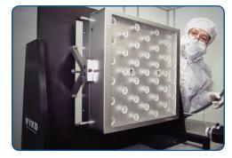
mirrors was fabricated, assembled, and tested at the University of Rochester's Laboratory for Laser Energetics and installed and successfully used on NIF to correct wavefronts for the first beams sent to target chamber center.
