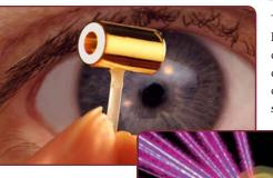
A NIF Hohlraum This tiny gold cylinder is a hohlraum designed for use during ignition experiments.
