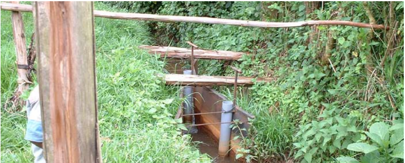
A simple turbidity monitor helps assess the success of upstream interventions to control erosion and runoff, with the hope of preventing a recurrence of damaging floods. (East Africa.)
