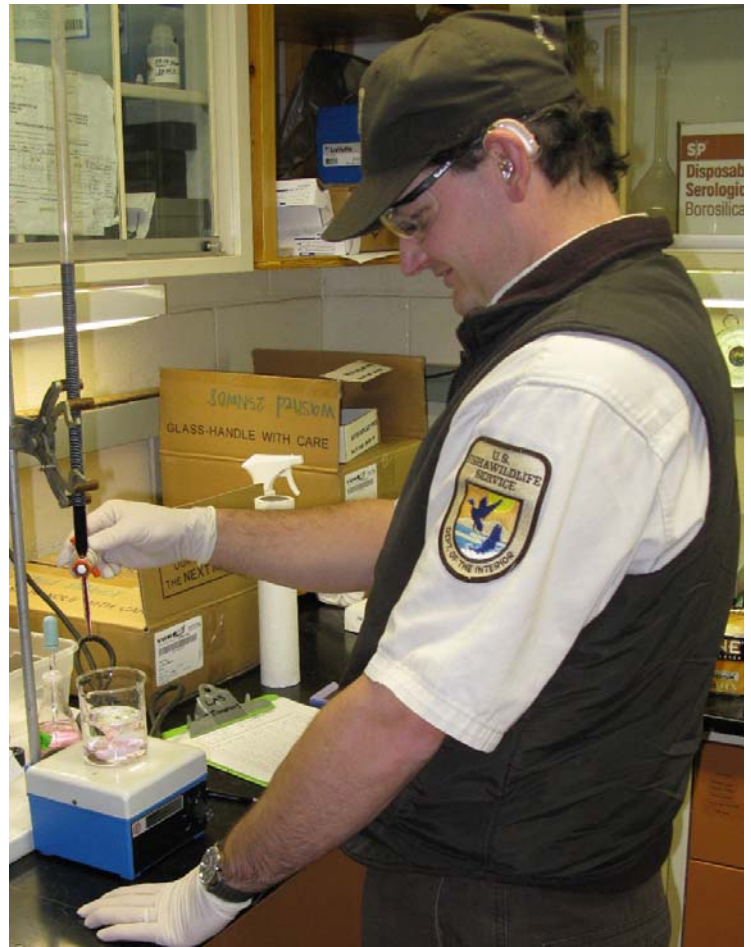
-USFWS Biologist Nick Grueneis titrates a sample of treatment water to check its concentration as part of a study to determine the effectiveness of hydrogen peroxide to control Gyrodactylus on cultured brook trout.
