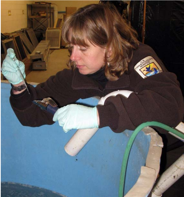
-USFWS Biologist Carey Edwards uses a refractometer to check the salinity of a salt bath for brook trout as part of a study to determine alternate treatment methods for the parasite Gyrodactylus at the Iron River National Fish Hatchery.
