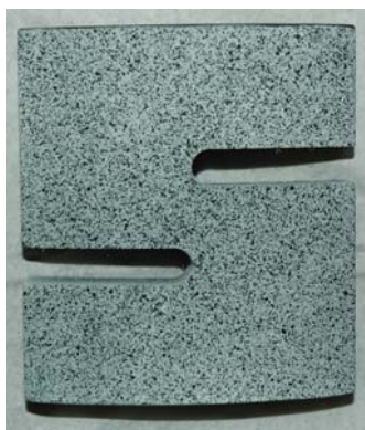
Figure 3. Composite shear specimen from section of a Mk82.
