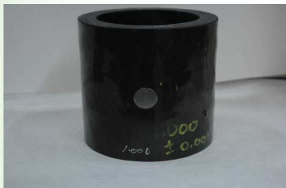
Figure 1. Fiber composite compression cylinder with 1.0-in.-diameter pin.
