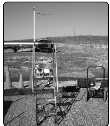
“Safety First” - The safety of site workers and the public (DuPont employees) is the team’s number one priority during site investigations. The team sets up exclusion zones to limit access to the drilling/work areas and monitors air and dust for organic vapors and radiation.
