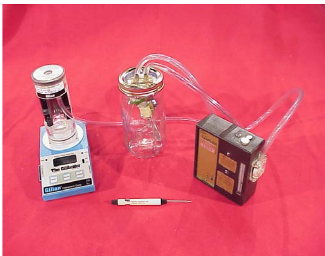
Figure 4-4. Gilian Gilibrator Set-Up for Calibration (Respirable Dust Cassette and Cyclone In-line)
