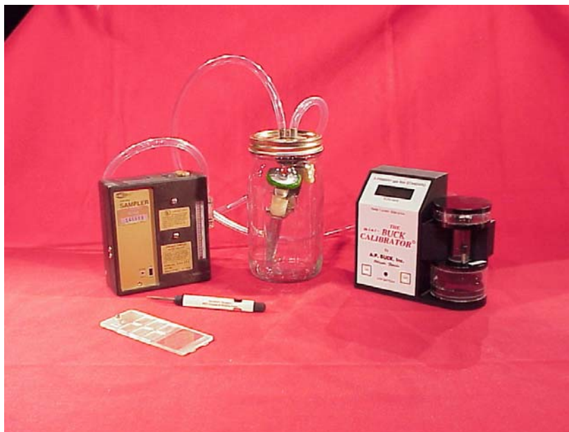
Figure 4-5. Mini-Buck Wet Bubble Calibrator Set-up for Calibration
