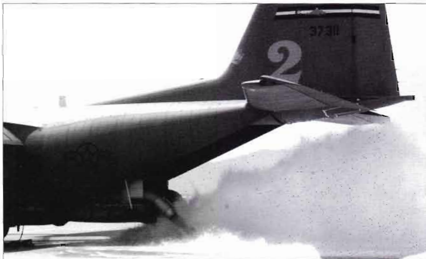
A Modular Airborne Fire Fighting System on a C-130 Hercules is flushed out with water before being refilled with fire retardant to continue airborne attacks against the Colorado wildfires.
