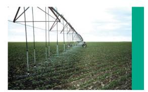
Converting from flood irrigation to a center pivot can result in an average water savings of 30 percent.
